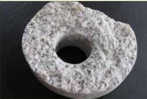
*A piece of Weardale Granite, from a borehole drilled at Rookhope by researchers at Durham University in 1960-61*
